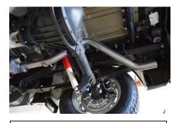
4. Install supplied 2-1/2" band clamp(Item I) onto inlet side of passenger side over-axle pipe(Item C) and install onto outlet of muffler. Install hanger into factory rubber grommet hanger. Tighten with allowance for adjustment
